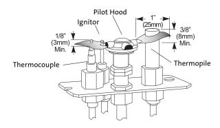
Figure 25. Correct Pilot Flame Pattern
